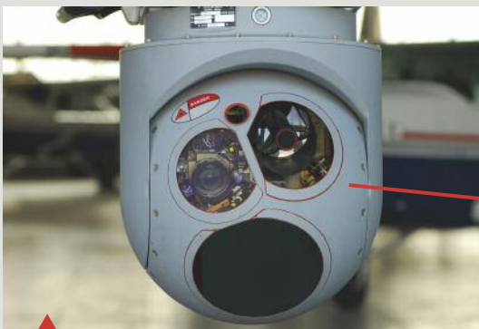
MX-15 turret containing an MX-15HDi sensor camera, once located under the left wing, is mounted in the fuselage on newer aircraft.
